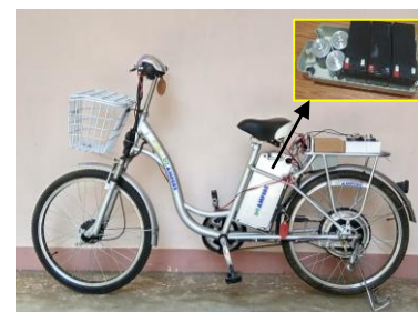
Hybrid (super capacitor assisted and lead acid battery powered) E-bicycle.
